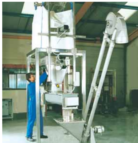
AMC designed for handling titanium dioxide. The aero mechanical conveyor is the only effective method of handling this type of product.
