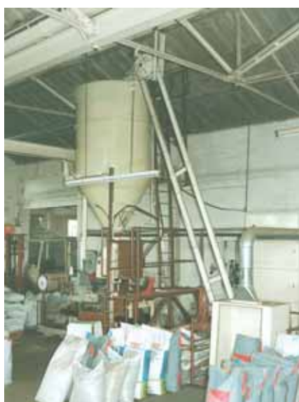
An aero mechanical conveyor elevating chemicals. Discharge heights can be specified to suit individual specifications.
