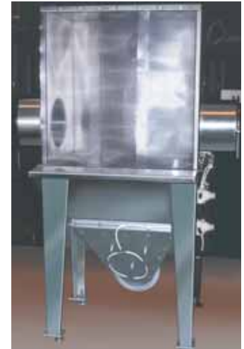
In sack emptying operations, a dust hood is often necessary. A sack compaction device may also be supplied.
