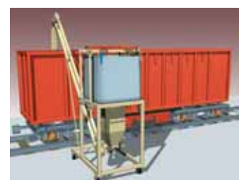
Bulk bag discharger and AMC loading rail car.
