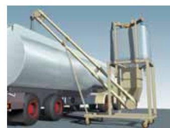
Bulk bag discharger and AMC loading road tanker.
