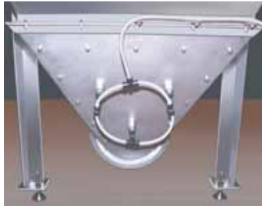
Inlet chute with aeration device
