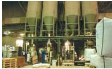
Filling materials in bulk bags and sacks in a minerals processing plant.
