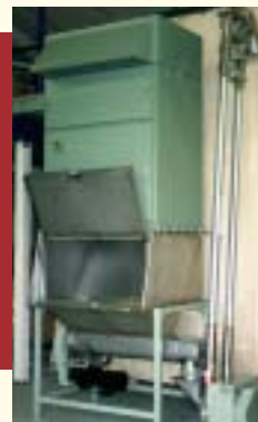
Vertical conveyor feed from sack tip station with screw feeder outlet and integral dust extraction system.
