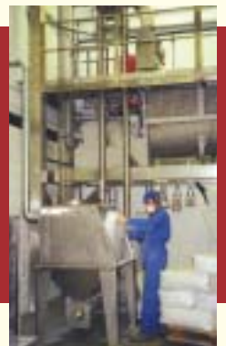
Manual sack tipping into mixer using vertical conveyor and integral feed screw.
