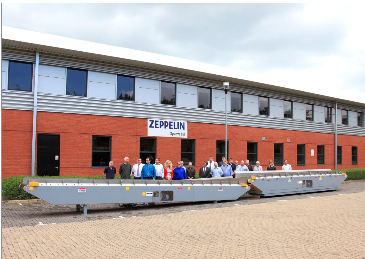
8m polymer scale (right) and 9m mixer charge conveyor outside Zeppelin's Nottingham site.
