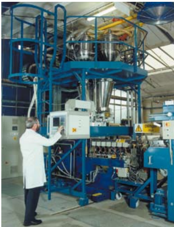
K-Tron PCS central receivers refilling K-Tron feeders on a twin screw extruder.
