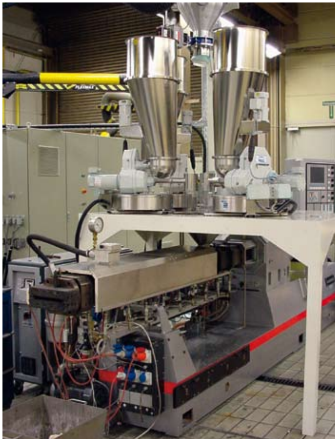
Modular loss-in-weight feeders arranged over an extruder
