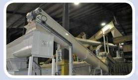
Tubular & Screw Conveyors: Widths from 2m to 8m single and dual column with capacities from 8 to 150tph. All Perry Grain Driers are designed and manufactured in the UK and are designed to BS6399 for wind loading and BS5950 for structural strength with a fully galvanised construction. Grain column is manufactured from 2mm thick galvanised steel and has a completely ledge free design to reduce dust and straw residue.
