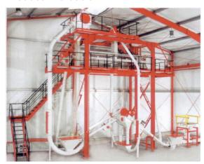
When conveying bulk materials, it is always best to consider a trial of the product. The system above is a part of the extensive test facility at Schrage Rohrkettensystem HQ in Friedeburg, North Germany. Customers are always welcome to visit the company and the large test hall can prove most applications. We also have a smaller demonstration unit in the UK which demonstrates the principles of the system.
