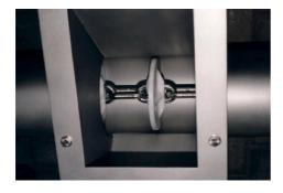
The conveyors consist of a series of disks attached to a chain. This assembly is drawn through a tube, which completely encloses the conveyed material. The chain runs as an endless loop and is drawn through the tubes by a rotating drive sprocket, fitted at the head end of the conveyor.
