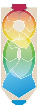
The Gyratory Reciprocating Motion gradually diminishes along the length of the machine to an elliptical path and finally to a nearly straight line motion at the discharge end.
