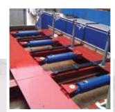
The Push Floor discharge machine can be used in three basic configurations.
