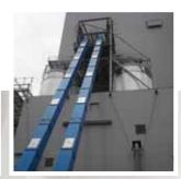
The Saxlund Chain Conveyor is a continuous operating conveyor enclosed within a bolted rectangular cross-section casing. It may be arranged horizontally or inclined with bends to suit the application.
