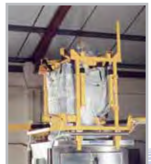
4. Bag Massagers at each corner assist flow and ensure total emptying.
