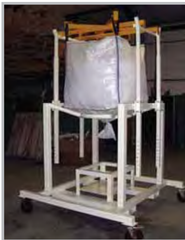
Customised Model T1 mounted on a wheeled frame that can also be moved by a forklift truck.
