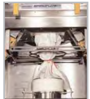
2. Spout pulled through the discharge dish (pinch bars open).
