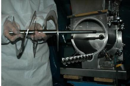
Lancashire-based Trantec Solids Handling Ltd, a leading provider of powder handling equipment to the bulk solids handling industry have introduced innovative new features allowing easy-clean of Trantec's "M" Series metering screw feeders with almost complete dismantling in less than 5 minutes.
