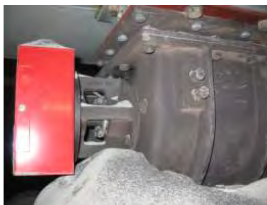
Rotary valve with leaking shaft seals
