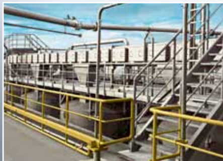
Gas-tight horizontal pendulum bucket conveyor
