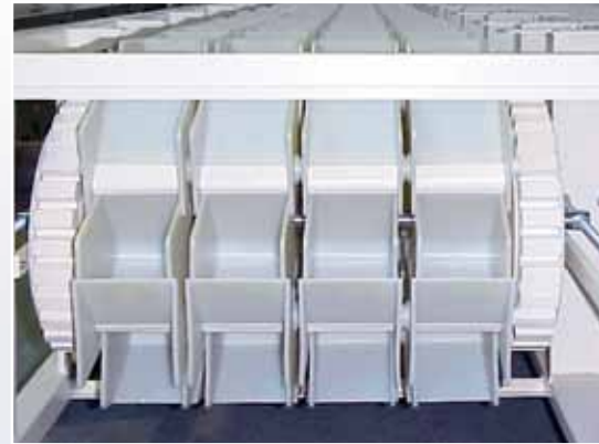
Multiple bucket belt at the tensioning unit
