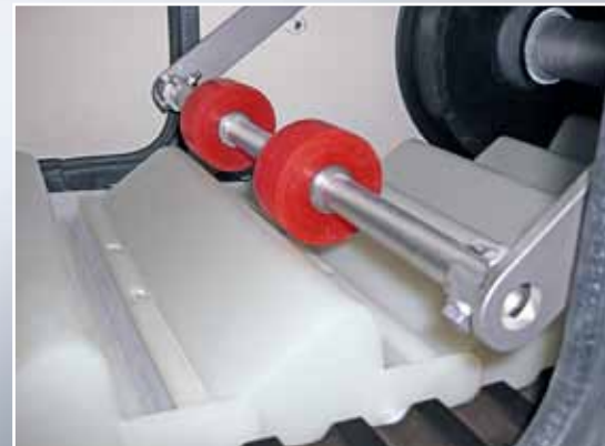
Pendulum bucket knocker to assist product discharge
