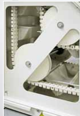
Transition from horizontal to vertical conveying
