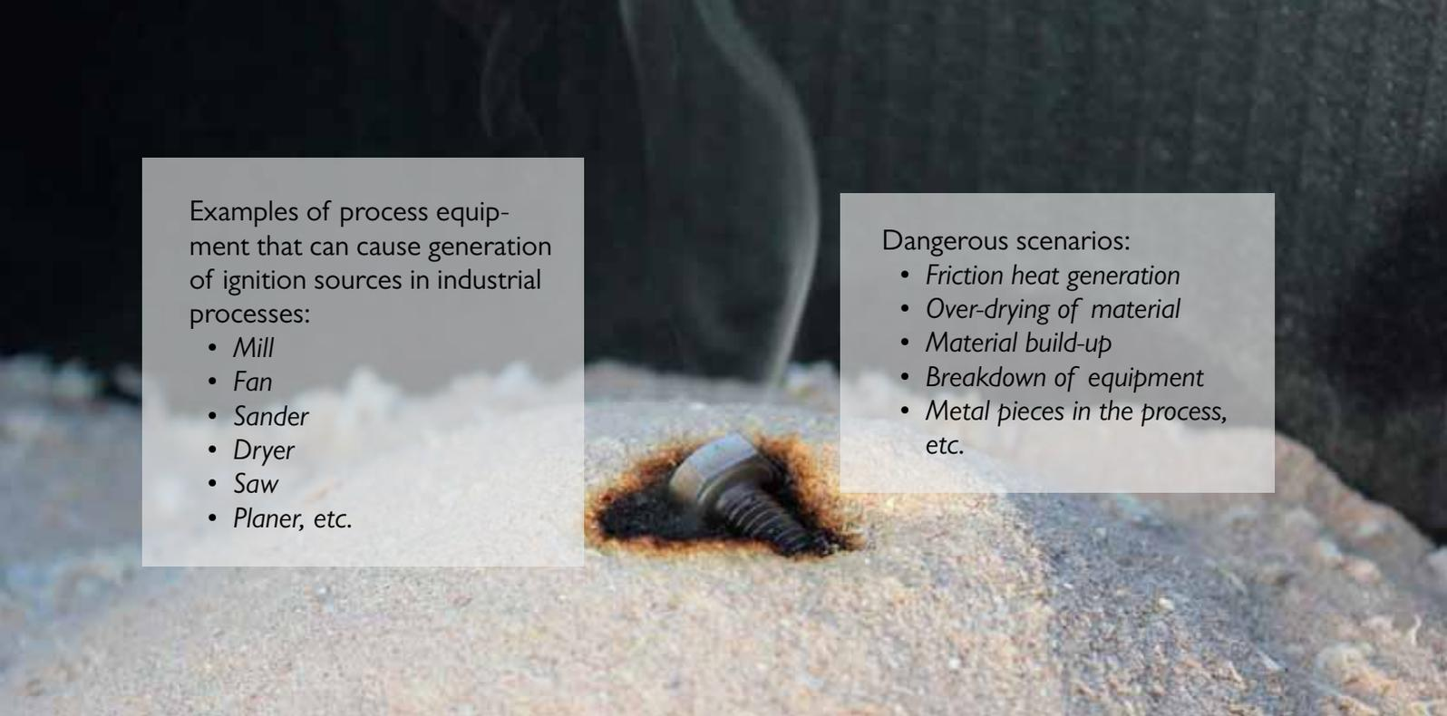
Examples of process equipment that can cause generation of ignition sources in industrial processes:
