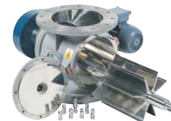
HDER Rotary Valve (easy-clean option) with fully demountable, deep-scalloped, sealed-end rotor for hygienic applications.
