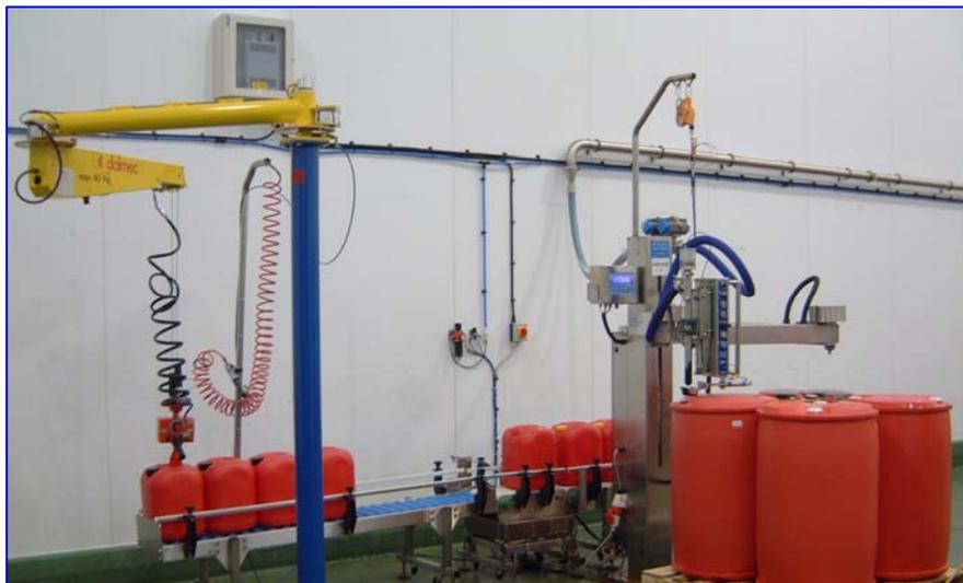
caps. The full container is then removed from the conveyor and stacked on a pallet using a pneumatic powered lifting unit. Depending on the viscosity, the containers can be filled in less than 20 seconds, to a tolerance of +/- 10 g.
