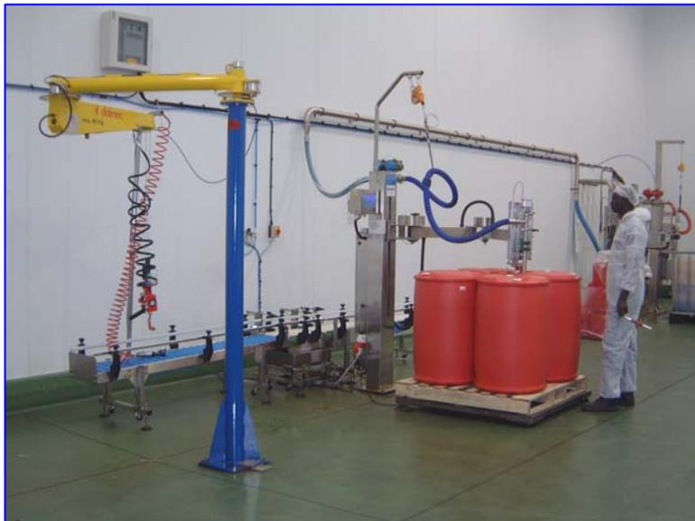
The Weightron Bilanciali system is based around a gravimetric StrongArm filling machine, which offers significant flexibility and versatility. The Healy Group's Operations Manager Mervyn Penson is very upbeat about the new system and as he explains: "The design of the line gives us the best of both worlds and allows us to accommodate the different filling requirements for the wide range of end customers. The new
