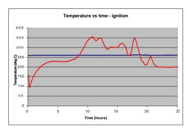
Typical 5 mm layer ignition temperature test trace for sewage sludge, showing ignition on a hot surface at 260°C
